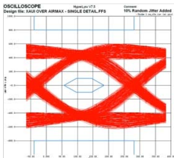
Figure 1. Eye Diagram for a XAUI signal across a total of 40 cm FR4 PCB, four vias and a mated pair of Airmax VS connectors. 10% random jitter was added in the simulation
