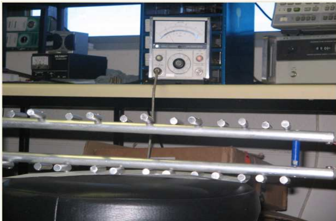
Figure 5.9 LPDA connected to the power meter
