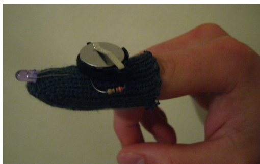
Figure 5.1: Photo of the LED system mounted on an index finger.
